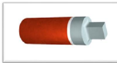
Fig 1: Photographic View of Resistance welding electrode
