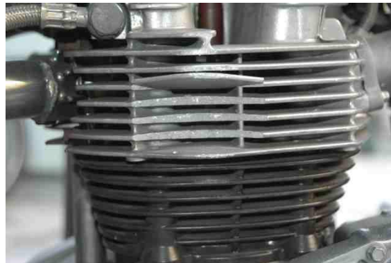
Fig.1.1: Two Wheeler Engine Cooling Fins
