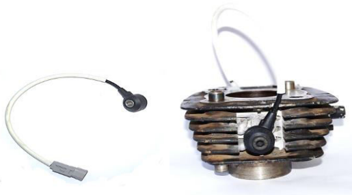
Fig. 7. Knock sensor & placement position
