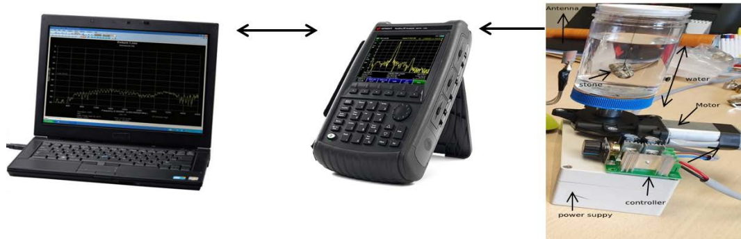
Fig. 5: Early detection process system for kidney stone
