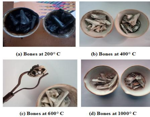
Fig 4: Calcined in a muffle furnace at different temperatures (200, 400, 600, 1000° C)
