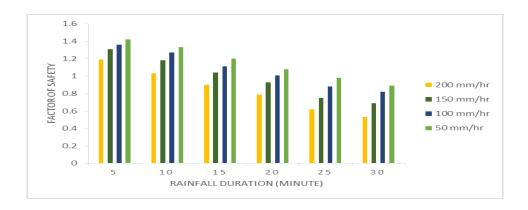
Fig. 4 Factor of Safety of Model Slope Angle 26.8<sup>0</sup> without Vetiver Plant for different
