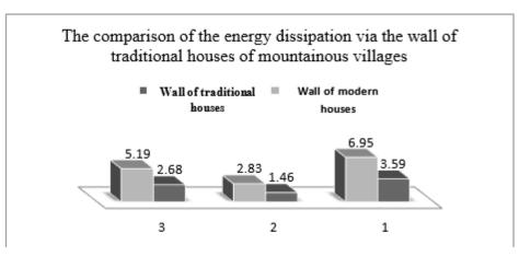
Chart 4- Comparison of the amount of energy loss via the wall of the studied (modern and traditional) samples of
