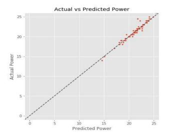
The X Axis of the graph represents the predicted power and the Y axis represents actual power. The pointed dots depicts the input values. Since the dots are closer to the central line of the graph, It makes clear that the results are accurate.
