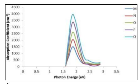
Figure 2: Absorption Coefficient for (PEO/PVA) Composites Thin Films of different Concentrations of CoCl<sub>2</sub>.
