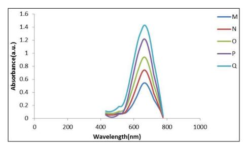
Figure 1: Absorbance for (PEO/PVA) composites thin films of different concentrations of CoCl2.
