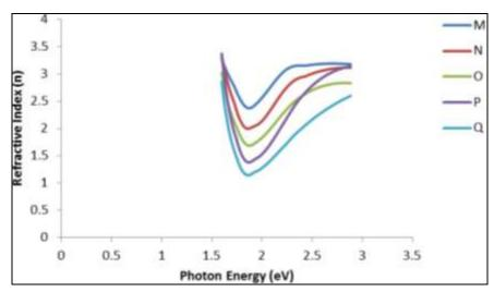
Figure 5: Refractive Index against the Photon energy (eV) for (PEO/PVA) composites thin films of different concentrations of CoCl<sub>2</sub>.
