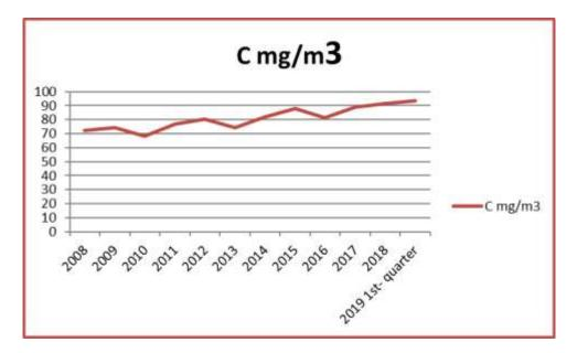
Figure 3: Concentration of Grain dust after Cleaning in the Elevator
