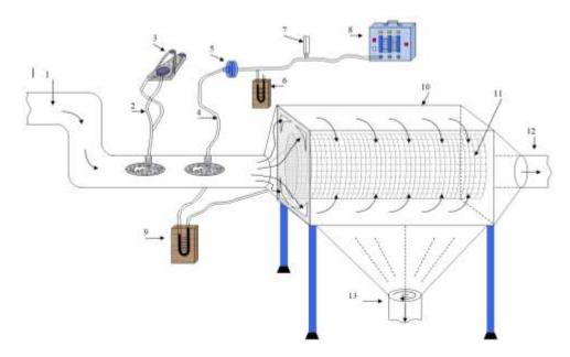
Figure 1: Energy-Saving Simple Dust Collector: 1 - Inlet Pipe; 2 - Pneumatic Tube; 3 Micromanometer; 4-Pipe for
