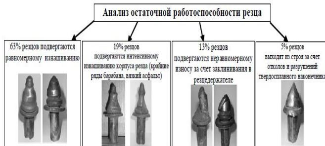
Figure 4 - View of the cutter of a worn cutter [13]
