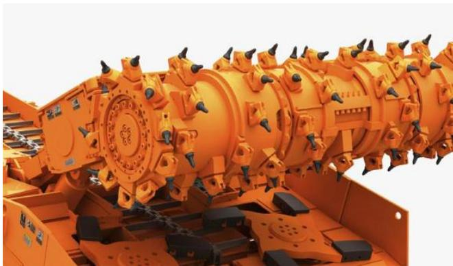
Figure 1 - The working body of a roadheader (analogue of the working body road miller).
