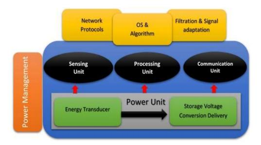
Fig. 1.1: Typical Sensor Node Architecture
