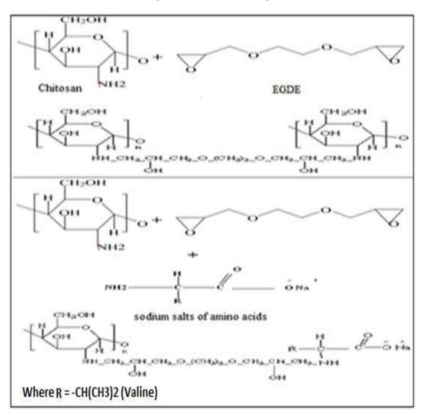
Scheme 1: Show possible cross linking mechanisms of chitosan with amino acids by using ethylene glycol diglycidylether (EGDE) to synthesis beads type C<sup>(27)</sup>
