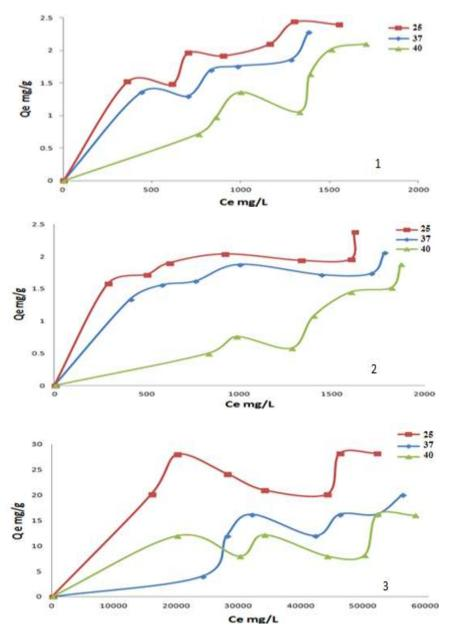
Figure 5: Show adsorption isotherms of (1=TC, 2=TG and 3=TP) on synthesisbeads surface (type C)from dilute serum at (25, 37 and 40 °C)
