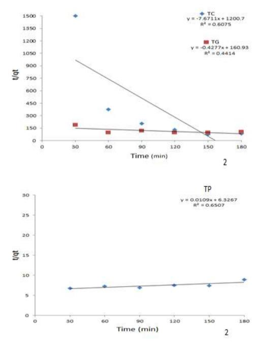
Figure 8: 1-pseudo first-order and 2-pseudo second-order for a adsorption process of (TC,TG and TP) on modified chitosan beads surface at 37°C
