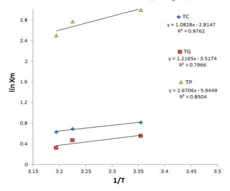
Figure 7: (lnX<sub>m</sub>) plotted against reciprocal absolute temperature for the adsorption of (TC, TG and TP)on modified chitosan beads surface
