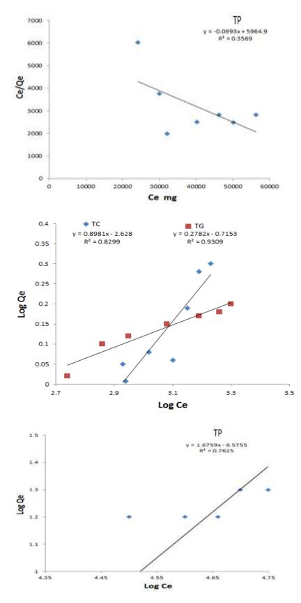
Figure 6: Langmuir and Freundlich adsorption isotherms for adsorption (TC, TG and TP)
