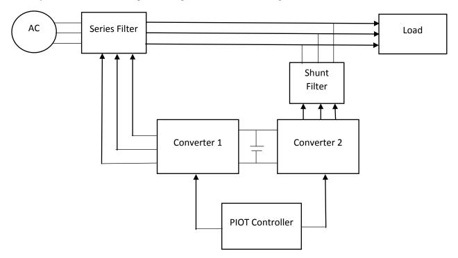
Figure 1: Proposed Block diagram
