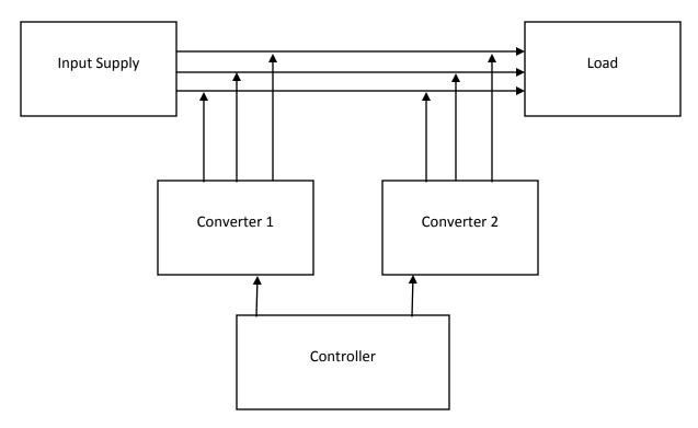
Figure 1: UPQC control Block diagram
