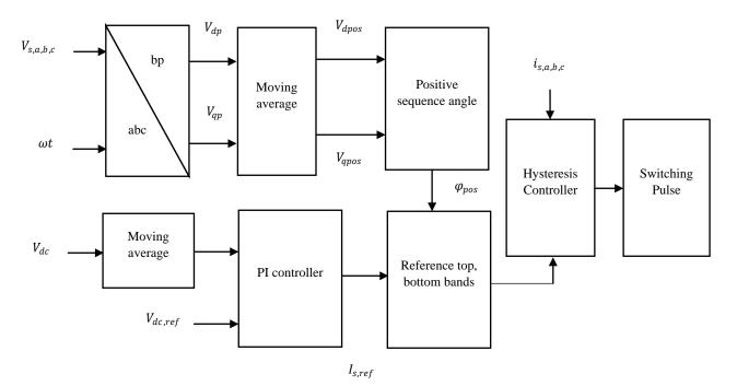
Figure 2: Shunt Active Power Filter
