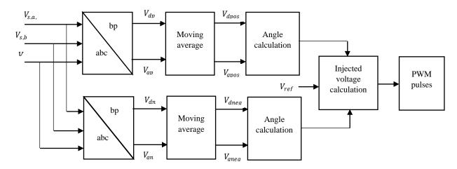
**Figure 3: Series Active Power Filter**
