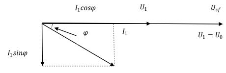
Figure 4: In-phase compensation Phasor diagram
