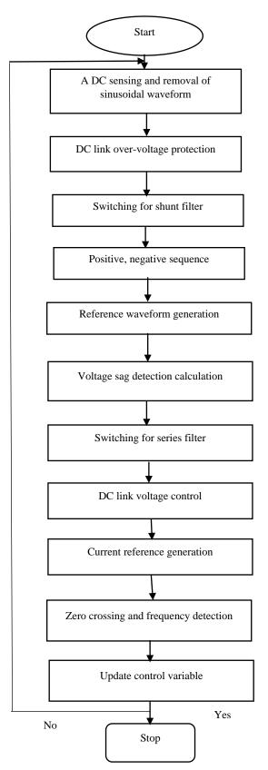
Figure 5: Proposed Power Impelling Optimization Technique(PIOT)Flowchart
